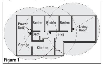
3. If the installation is for new constructions and you are working with 1/4" scale blueprints, use a seven inch string to represent the hose.
